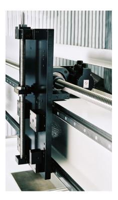
Accuracy in linear guides depends on many factors, including the trueness of the rail on which the runner block travels.
