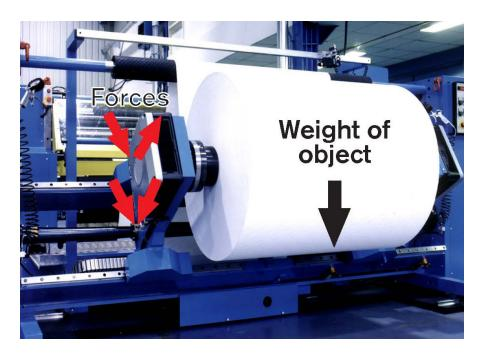
Axial or torsional loading, for example, may require wider or heavier-duty components than simple radial loading.
