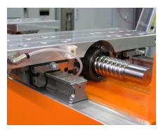
Ball screw and rail combinations like this provide a good balance of travel accuracy and load carrying capability, even with axial or torsional loading.
