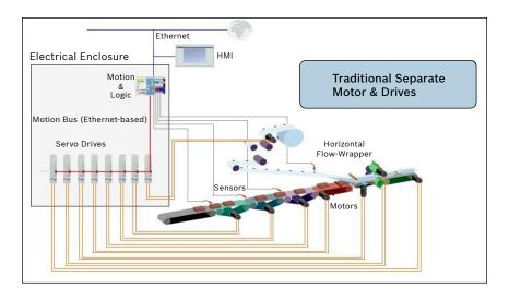
When selecting a traditional vs. integrated motor/drive servo system, consider factors such as space saving, overall cost, functionality and modularity.
