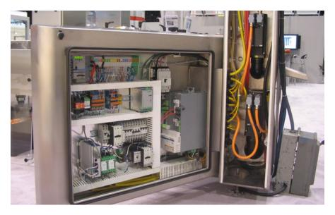
With integrated servo drive/motor technology, the drive electronics are relocated from the control cabinet and mounted directly on the motor at the machine.
