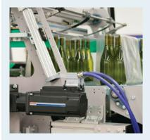
Integrated motor/drive systems are especially suited for modular machines, such as packaging equipment, where line extensions are added for different products. motor. The control cabinet is used to protect sensitive electronic elements from harsh factory floor conditions such as heat, vibration, static discharge and other factors.
